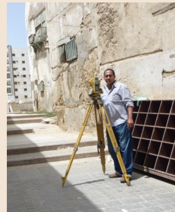
Surveying with Topcon GTS 702
