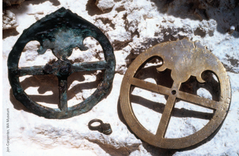
The pair of bronze astrolabes, Dutch navigational instruments from the Batavia wreck used for determination of latitude. The left-hand astrolabe had been exposed to the full brunt of the surf on Morning Reef, Abrolhos Islands, for 350 years; the right-hand astrolabe was in pristine condition, having been buried in an iron cannon ball corrosion matrix, which protected it from corrosion by galvanic action.
