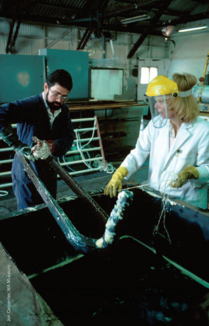
Molten wax impregnation and consolidation of heavily corroded bronze rudder pintle from the wreck of the American China Trader Rapid (1811); Ian MacLeod and Jennifer Edwards, intern from Australian War Memorial. The microcrystalline wax stops moist air getting to the extensively corroded object and causing accelerated decay. Analysis of the corrosion processes showed the pintle had been buried in 25–30 cm of coral debris.
